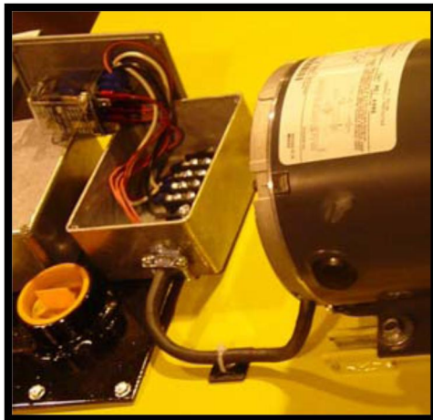
Terminal Block inside Electrical Box
