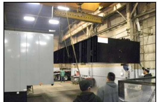
*A sub base tank is moved into position prior to mounting of the enclosure at the Tramont Heavy Lift Facility.*
